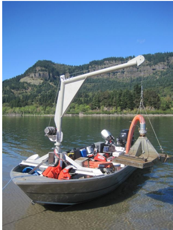
Figure 1. Diagram (left) and photo (right) of deepwater electrofishing device and boat to be used by USFWS to survey for Pacific lamprey ammocoetes in the area to be dredged.
